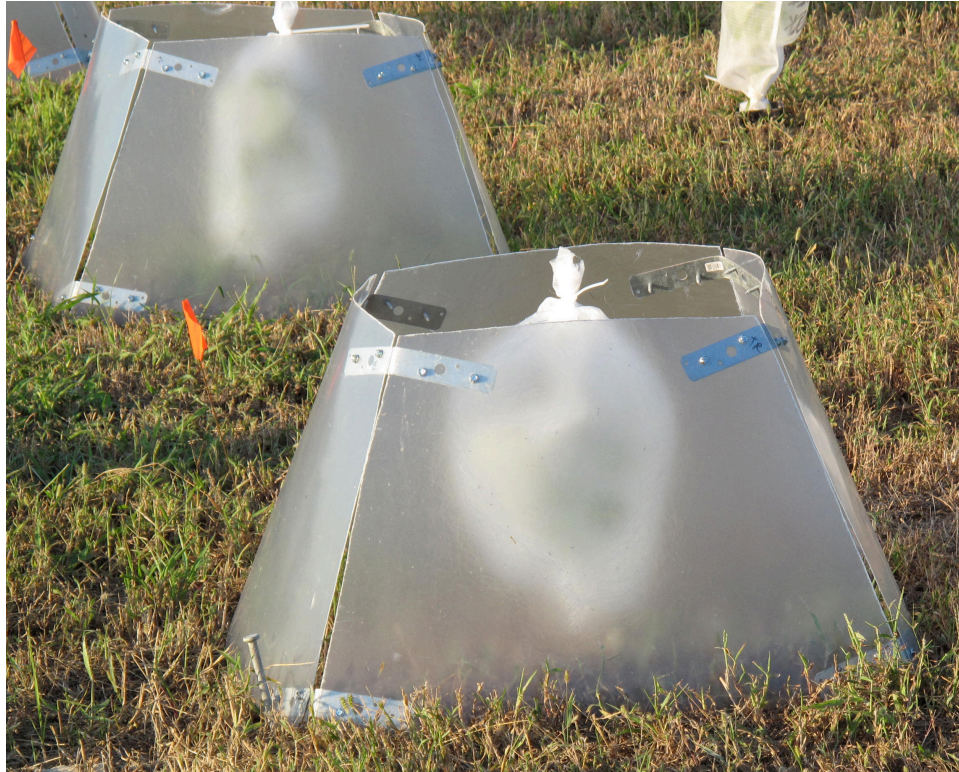
Figure S1: Open-top chamber (OTC) used to raise temperatures in the field experiments. In the center of the OTC, a single soybean plant was placed. The plant was enclosed in a mesh bag to prevent larval escape.
